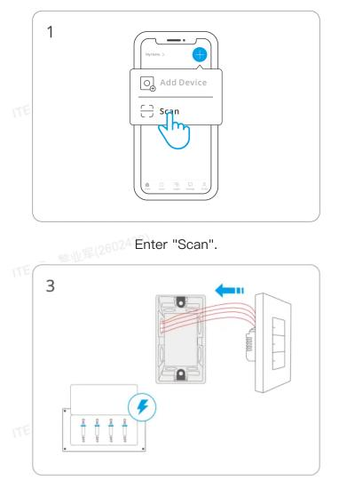
Install the device into the mounting box first, then power it on.
