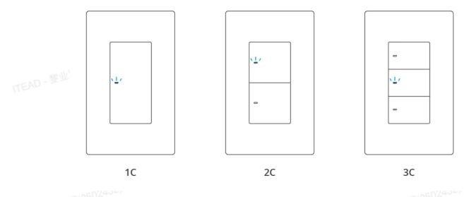
() The device will exit the pairing mode if you do not operate it within 3mins. When you want to enter the pairing mode again, long press the any button on the device for 5 seconds until the signal light "flashes slowly" and release.
